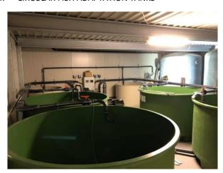
VASG's Circular tanks are manufactured with base or without base, depending on the size of the diameter. Large diameter tanks are assembled by flanges. We offer demand based options in different diameters on concrete floor.
